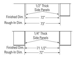
Note: 1/2" thick side panels shown. Side panels can be any thickness. Add side panel thickness to outside trim width (36" or 72" for two models) to calculate the rough-in dimension. The leading (front) edge must be finished to match surrounding cabinetry.
